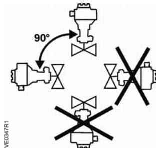
**Figure 1. Acceptable Outdoor Mounting Positions with Weather Shield.**
