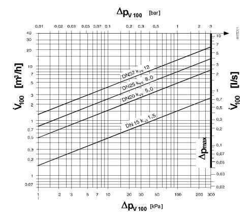
$\Delta p_{v100}$  = differential pressure across the fully open valve and the valve's control path by a volume flow  $V_{100}$
