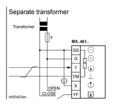
Terminal assignment for controller with 3-wire connection
