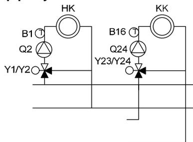
The cooling and heating circuits draw their cooling/heating energy from separate primary circuits.
