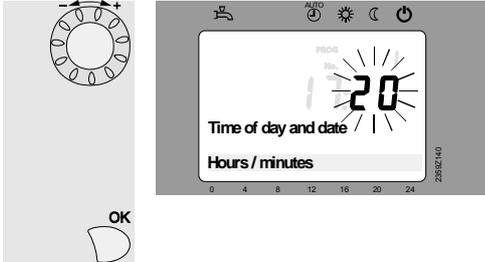
The display shows the minutes flashing. Turn the setting knob until the minutes of the time of day are correct. To confirm, press OK.
