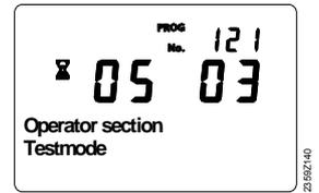
The digits on the left show telegrams that have been sent, the digits on the right telegrams that have been received. The test will be ended after 24 telegrams. The test is considered successful when at least 50 % of the telegrams sent have been received.
