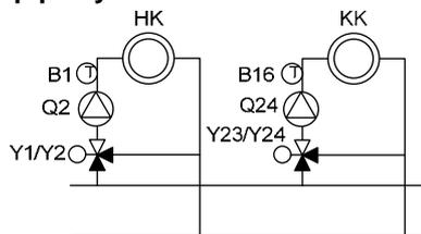
The cooling and heating circuits draw their cooling/heating energy from the same primary circuit.
