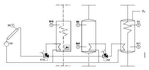
Solar storage tank and swimming pool charging via diverting valves with 2 collectors
