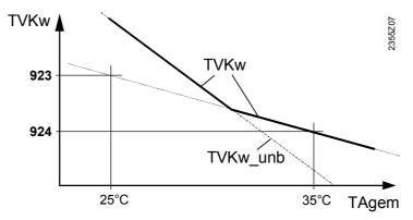
TVKwFlow temperature setpoint for cooling (with low limit control)TVKw\_unbFlow temperature setpoint for cooling (without low limit control)TAgemComposite outside temperature
