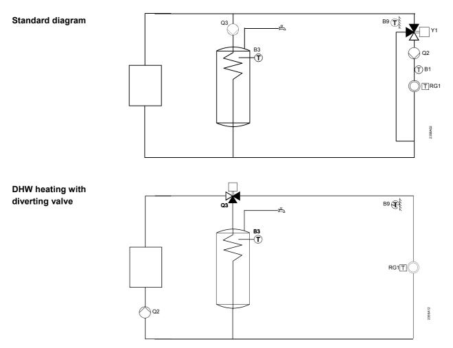
Heating/cooling via diverting valve
