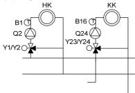
The cooling and heating circuits draw their cooling/heating energy from separate primary circuits.
