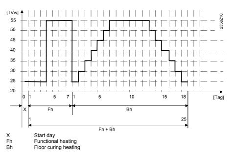
Floor curing setp The flow temperature setpoint for the "Manual" floor-curing function can be set separately for each heating circuit.
