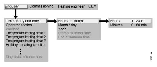
Setting the structure "Heating engineer"
