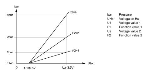
Voltage value 1 Function value 1 Voltage value 2 Function value 2 • Example of relative room humidity 10V
