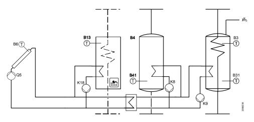
Solar storage tank and swimming pool charging via charging pumps with 2 collectors
