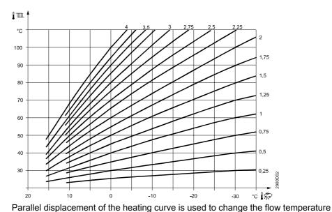
Heating curve displacement
