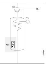
DHW tank with external heat exchanger, charging pump, intermediate circuit pump
