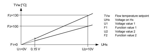
If the input signal drops below the limit value of 0.15 V, the heating demand is invalid and therefore has no effect.
