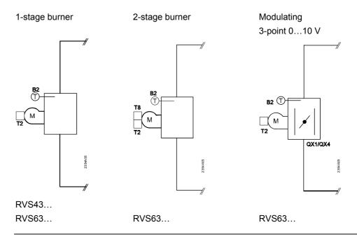
Burner without boiler sensor
