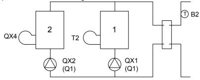
Due to the temperature differential between boiler temperature setpoint and boiler temperature sensor B2 (common, mandatory cascade flow temperature sensor), switching on / off of the lag boiler (release and reset integral) takes place according to the control of a 2-stage burner. The same parameters are used.
