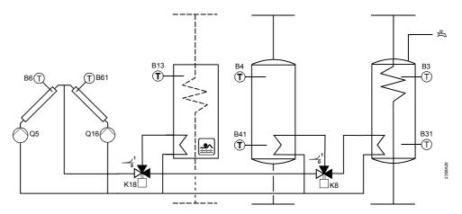
Solar storage tank and swimming pool charging via charging pumps with 1 collector
