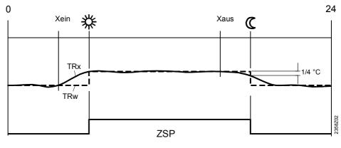
XeinSwitch-on time shifted forward in timeXausSwitch-off time shifted forward in timeZSPTime switch programTRxActual value room tempTRwRoom temperature setpoint
