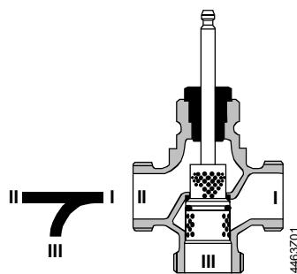
Guided perforated plug which is integrated in the valve stem.
