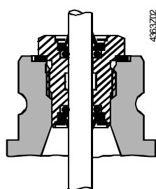
Replacement for EPDM-O ring sealing gland made from dezincification-free brass, including flat seal made from copper, for cooling water, chilled water, low temperature hot water, high temperature hot water, saturated steam, and brine –25...+140 °C
