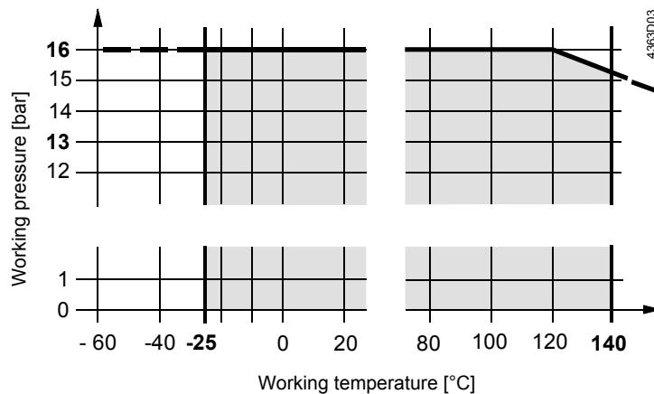
Working pressure staged as per ISO 7268 and EN 1333
