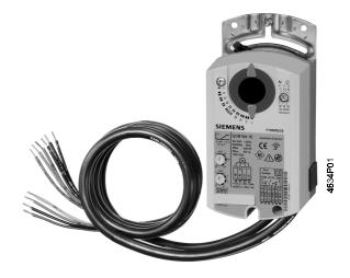
Electric motor-driven actuators, modulating for DC 0...10 V control signals, nominal torque 5 / 10 Nm, AC 24 V operating voltage, self-adaptation of the rotational angle range, DC 0...10 V feedback signal for position indication, mechanically adjustable working range between 0...90°, pre-wired with connecting cables of 0.9 m. Type-specific variations with adjustable control signal for offset and span and with adjustable auxiliary switches for supplementary functions.
